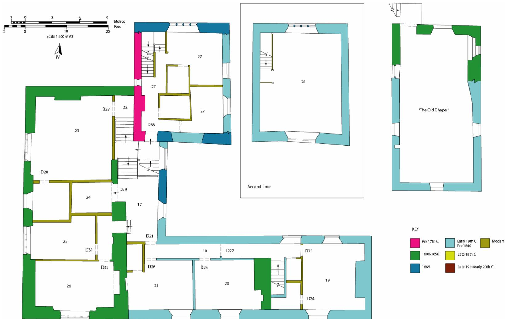
Figure 18: First and second floor plans showing the developmental phasing.
