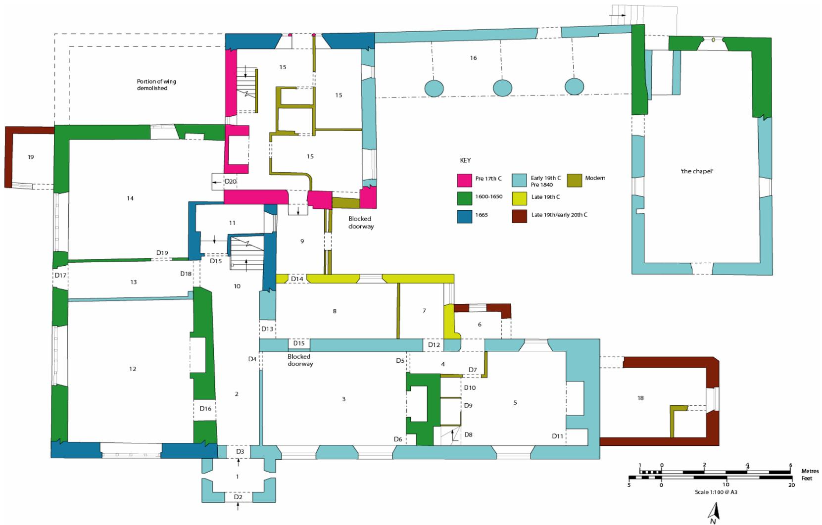
Figure 15: Ground floor plan showing developmental phasing.
